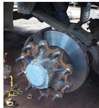
A brake disc is shown here before and after the skimming process. Skimming truck discs reduces time off the road, since the disc can be skimmed in situ within just 20 minutes, saving you time and money.
