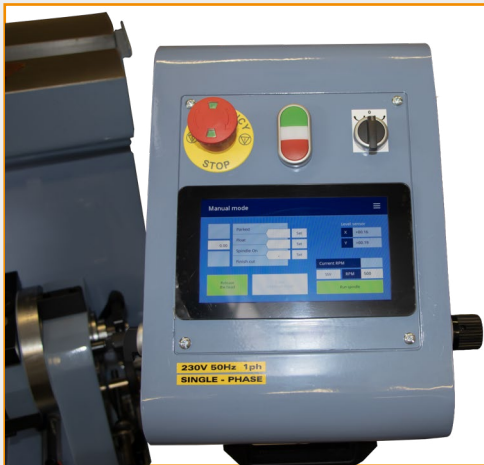
The touch screen panel with SMART AID guides the operator through each step, while the large front handwheel and micrometric side knob keep direct control of spindle downfeed.
