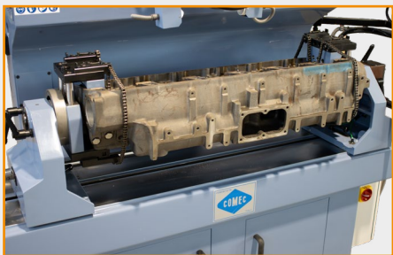
360 degree Rollover fixture assures a complete accessibility to all sides of the cylinder head. The clamping process is very quick and assures high sturdiness. The levelling procedure is definitely simple thanks to the fine adjustment knob.
