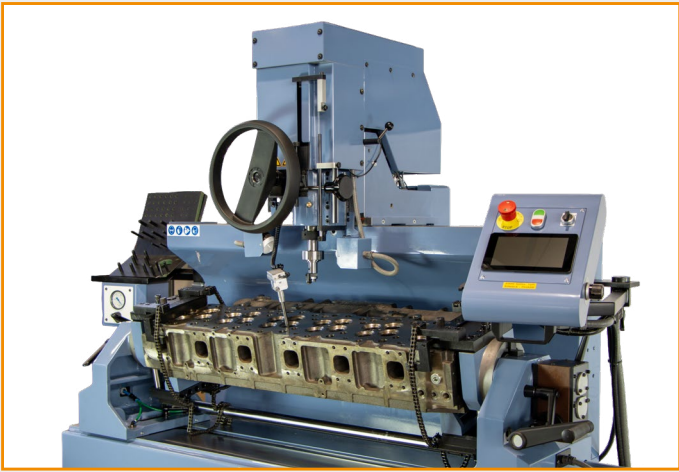
Spindle Workhead extremely sturdy mounted on air cushion to provide a light and quick positioning.
