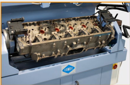
360 degree Rollover fixture assures a complete accessibility to all sides of the cylinder head. The clamping process is very quick and assures high sturdiness. The levelling procedure is definitely simple thanks to the fine adjustment knob.
