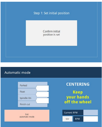
The touch screen panel with SMART AID guides the operator through each step, while the large front handwheel and micrometric side knob keep direct control of spindle downfeed.
