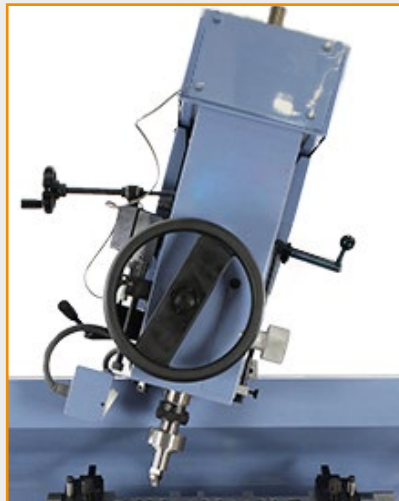
The touch screen panel with SMART AID guides the operator through each step, while the large front handwheel and micrometric side knob keep direct control of spindle downfeed.
